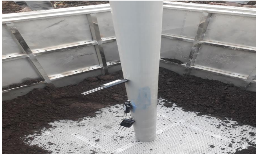
Plate 7. Placing of mesh and soil moisture sensor at the bottom of inner tank to prevent washing out of soil through drain
