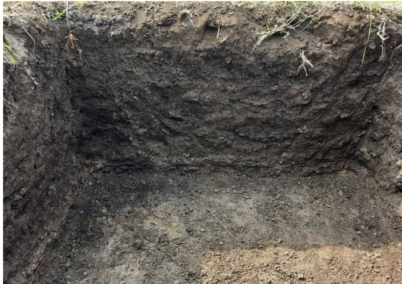
Plate 4. 1 m × 1 m pit from which soil was excavated layer wise to fill in inner tank of Lysimeter
